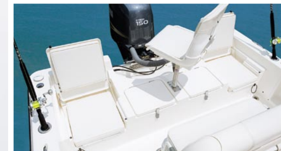
Rear casting deck provides additional seating with port and starboard flip-up seats that fold down flush when not in use.
