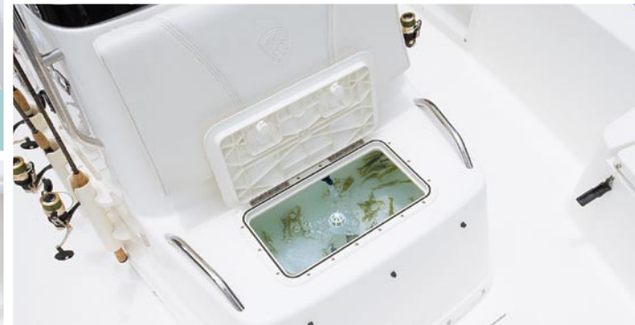
Console seat reveals baitwell with PowerStream® Venturi aerator.
